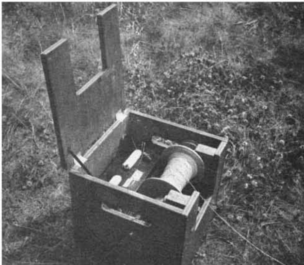
Gas powered winch offers unlimited power and flexible speed. Plate bolted to head holds throttle and clutch arm. Keep your arm off that plug!!!
