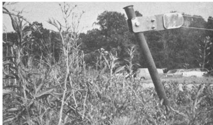
Pulley on stake reverses towline direction. Allows winch operator and glider launcher to be at same end of field. Also makes solo winch launch possible.
